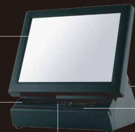
System and printer status LEDs, power switch, brightness control buttons
